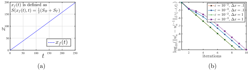
Figure 16: Convergence study for the hysteresis model. The parameters are S_B = 0.2 , S_T = 0.6 , \Delta x = .1 , \Delta t = 10^{-3} , \varepsilon = 10^{-3} unless specified otherwise.
